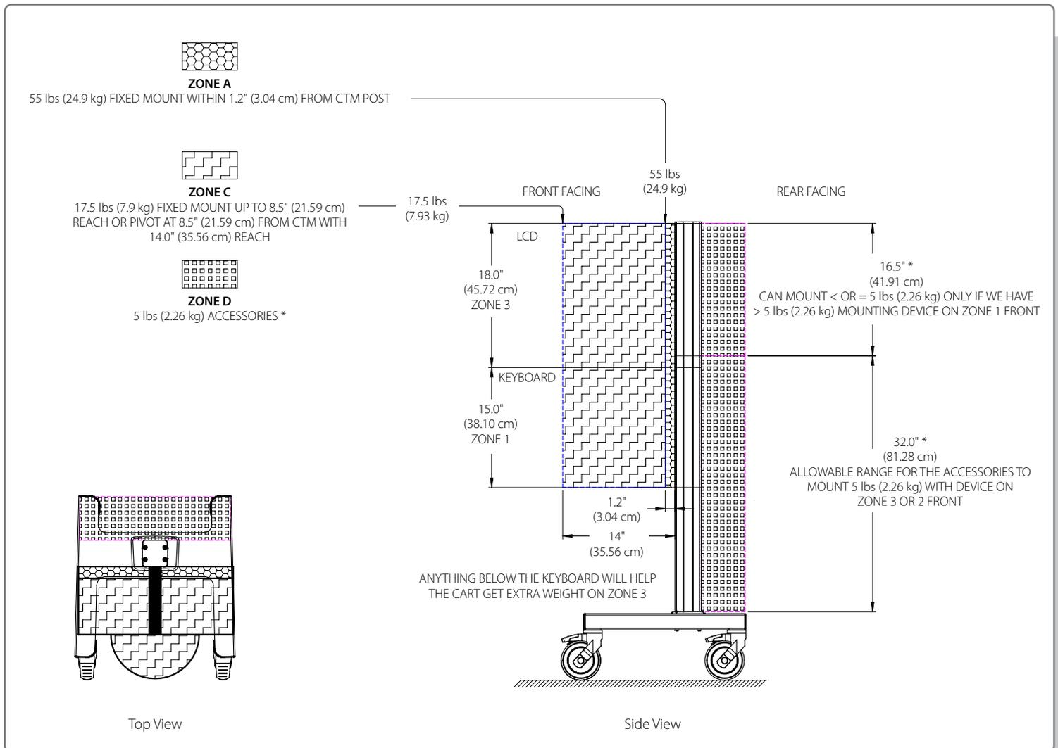
Figure 5: Load Rating With Zones (Swivel Mount)
