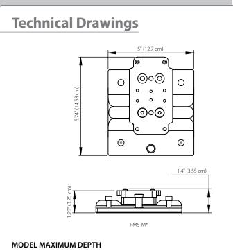
Back of adapter to front of plate (back of monitor) distance.
