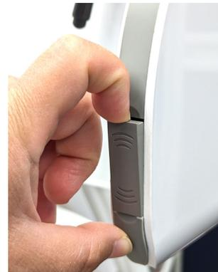
5. Insert the RFID Reader (USB dongle) gently and jiggle until the reader's USB connector aligns with the USB port inside the Sidekick Secondary Surface.
