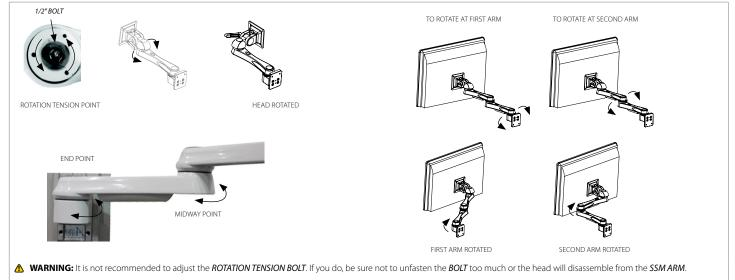
MARNING: Both arms have a 180° rotation. Ensure the proper clearance around the SSM ARM(s) to avoid collision.
