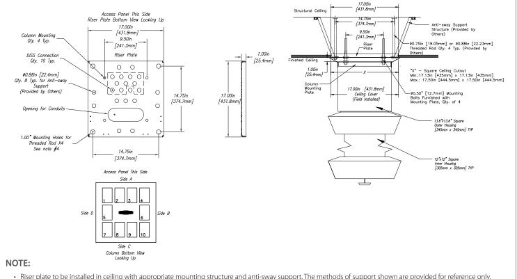
\* has place to be installed in ceiling with appropriate mounting structure and and sway support. The methods of support shown are provided to reference only
