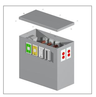
2. (Optional) Remove the access panel cover on the back of the floor pedestal by loosening the 6 screws attaching it to the floor pedestal.
