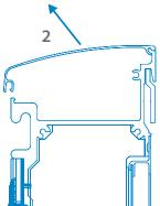
Remove lower cover by removing screws which hold it in place and lowering cover away from rear notch.
