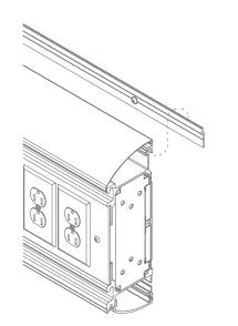
**NOTE:** End plate and cover removed in graphic for clarity. Do not remove!
