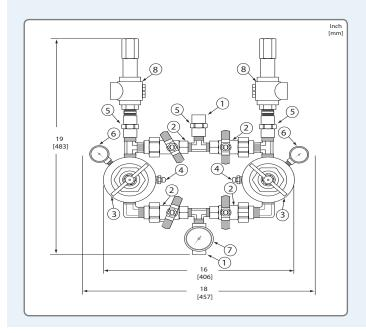
**Note:** Nitrogen requires a 300 psi pressure gauge and all other gases require 100 psi. The 1/2" dual line could be adapted to the 1", 2" or 3" supply line by the way adaptors at the in-let and out-let. (adaptors supplied by others)
