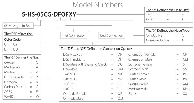
EXAMPLE: Oxygen 5' (60") Hose Assembly with Female DISS by Ohmeda Female Coupler with US Colors S-HS-05UO-DFOFC4
