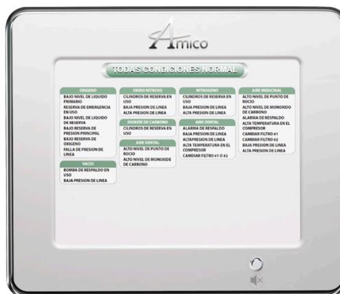
Alarma de Area Master Ethernet LCD Alert-4
