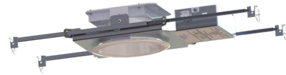
The **DL6 Recessed 6" LED Downlight** is designed for MRI suite applications. This low-profile, recessed application measures 3.9" in depth and comes equipped with either DC or Ethernet Wiring.
