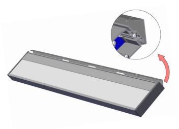
4. Wires must be run through the holes in the backplate and wired appropriately. Contact factory for custom wiring diagrams.
