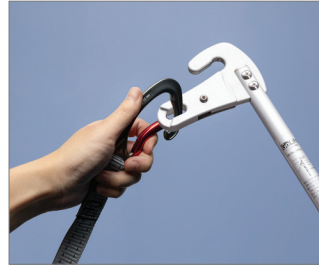
Closed carabiner attached to latch of the Reacher Bar
