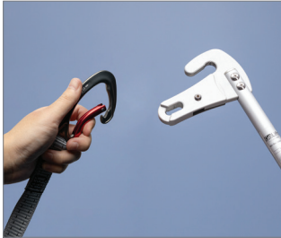
Open carabiner to attach in slot of the Reacher Bar
