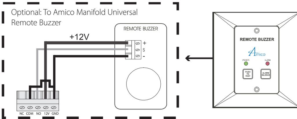
**NOTE:** Amico recommends max. 50 ft. to power up buzzer from alarm panel to power up the buzzer. More than 50 ft., a A3P-POWER-V4 is required to supply voltage for the alarm buzzer.
