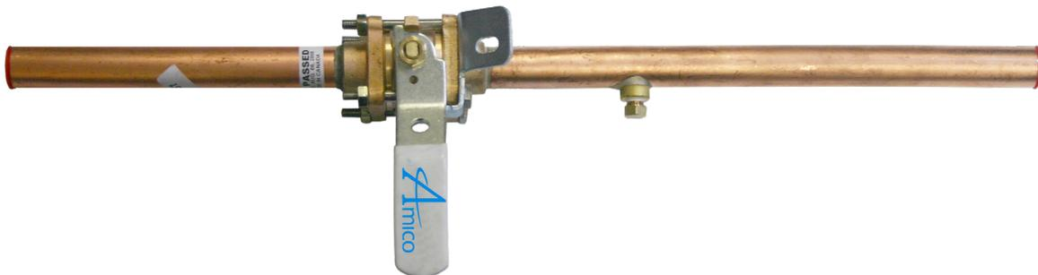
The Zone Valve Shut-offs shall be 3 piece, ball-type design with a brass forging body and a chrome plated, brass ball for sizes 1/2" to 2". Ball seats, stem seals and stem washer shall be reinforced Teflon (PTFE), with Viton stem and flange O-rings.
