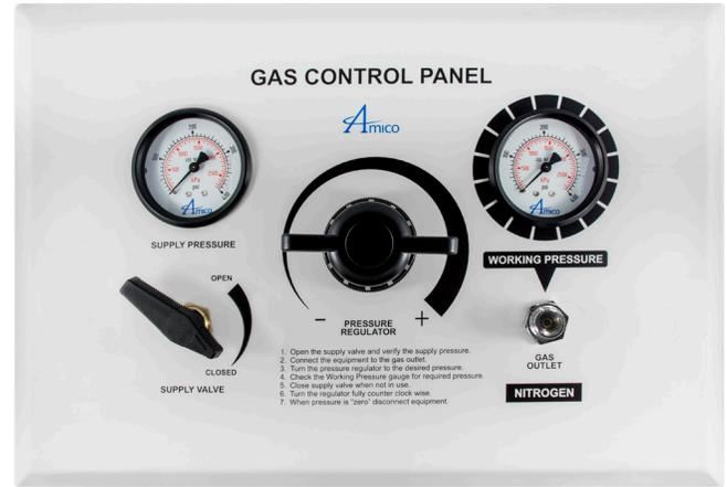
The DISS outlet shall be a Diameter Index Safety System (D.I.S.S.) For Air or Nitrogen Service Outlet or “Safety Swing Coupling” for pressures above 200 psi. The outlets shall be used for connection to pneumatic surgical tools.
