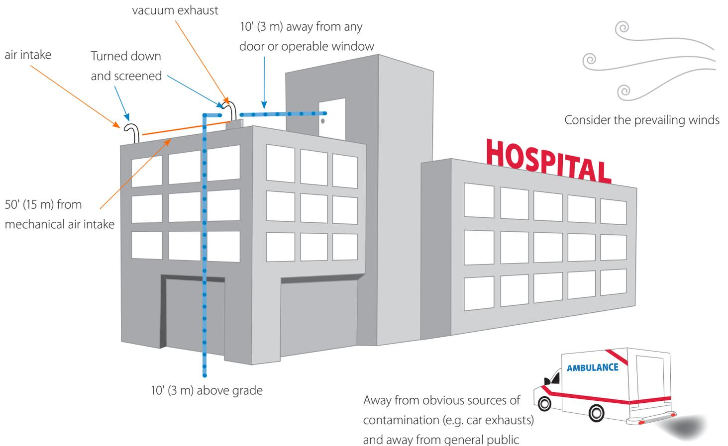
5. If the vacuum system is not already piped to the intended location, determine a routing for the exhaust piping and note it on the building drawings. Piping for medical vacuum systems shall be routed in such a way that it is not subjected to temperatures lower than 40°F (4°C). The exhaust shall be free of loops and dips in order to eliminate potential trapping of condensate or oil.
