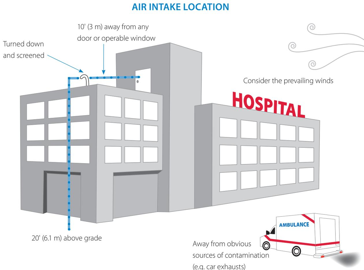
5. If the medical air system is not already piped to the proposed location, determine a routing for the intake piping and note it on the building drawings. Piping downstream of the compressor shall be routed in a manner such that it is not subjected to temperatures lower than 40°F (4°C).
