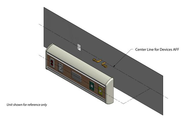
2. Mark a horizontal line for bottom of mounting bracket (to be installed later). This line is to be offset 4" (102 mm) above the center line for devices.
