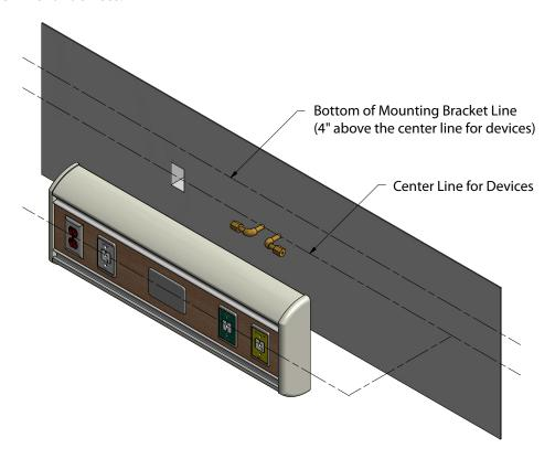
3. Using a stud locator, mark the location of any metal studs or blocking in the building wall that intersect the headwall mounting location.
