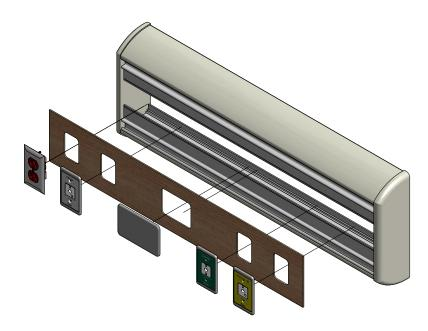
6. Verify the rough-in locations on the wall and align with the rough-in location in the headwall. Hang the headwall unit on the wall, over the mounting bracket.
